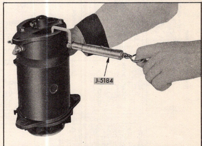
Fig. 7 Measuring Brush Spring Tension
