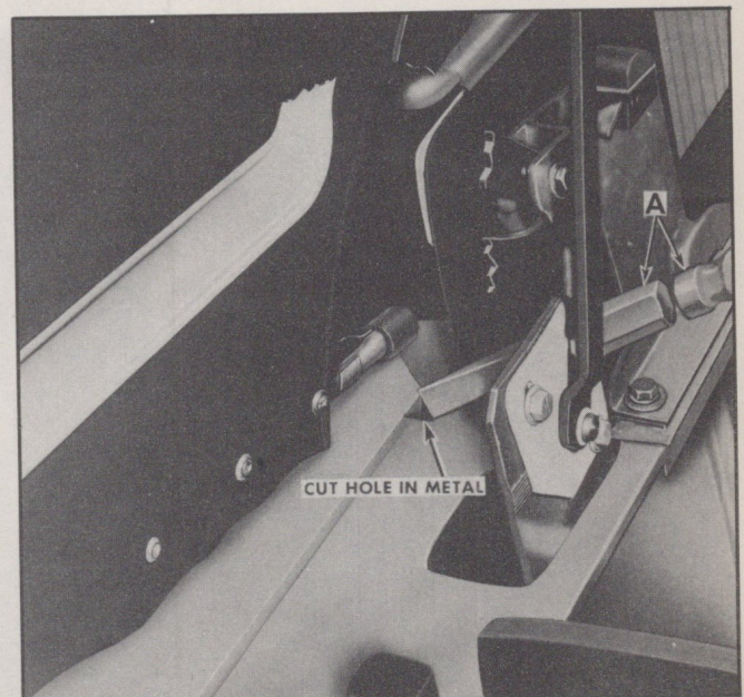
Fig. 7 Cutting Hole in Folding Top Compartment
