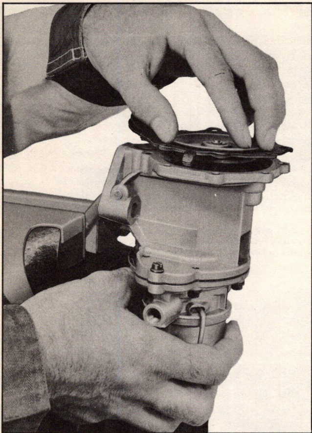
Fig. 7 Installing Vacuum Diaphragm
